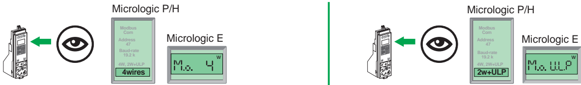
A Modbus RS 485 4-wire without ULP module
